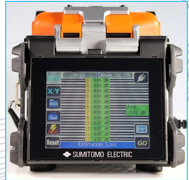
Fusion splice ribbon based cable to 12ct ribbon to LC fan-out
