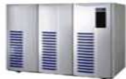
1993: EMC Symmetrix 16 MB DRAM, 1 GB global memory, 1 TB capacity
