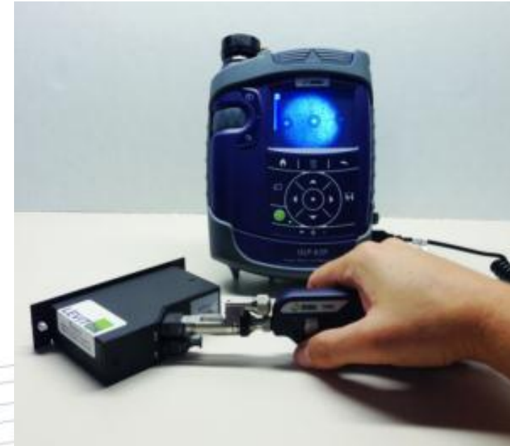
Bulkhead (“Female”) Inspection
