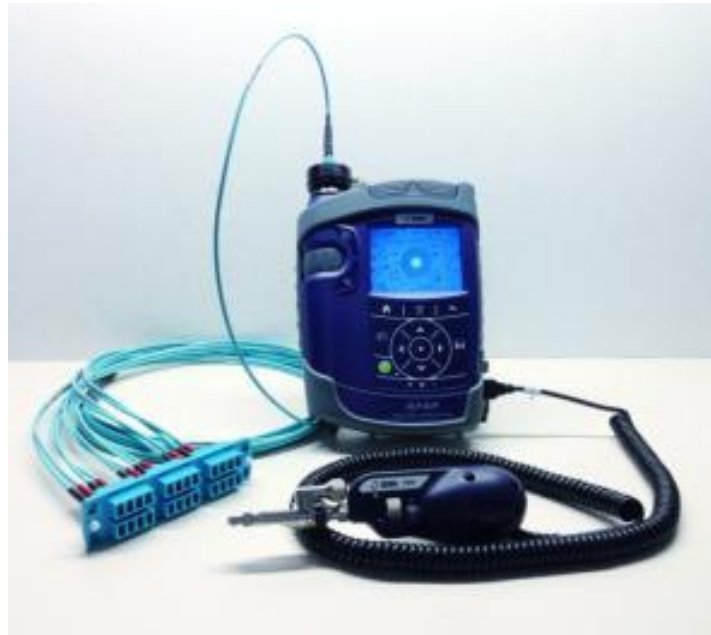
Patch Cord (“Male”) Inspection
