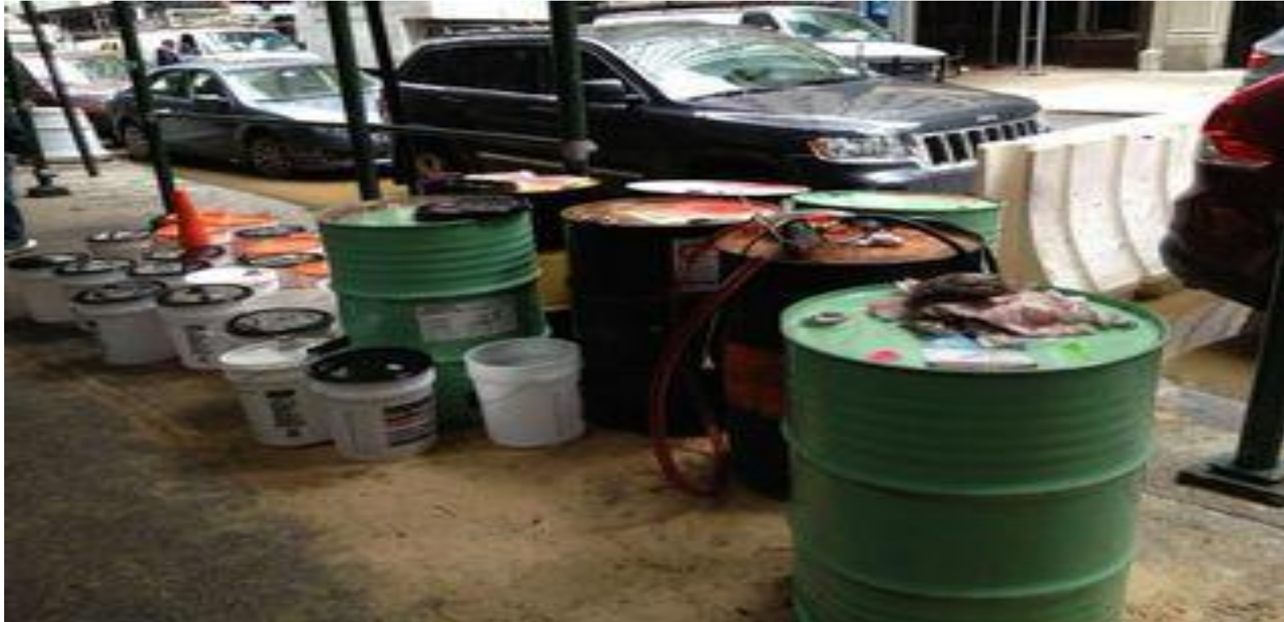
Example of Sandy Hurricane where fuel barrels are kept open in vulnerable state, raising risk of explosion
