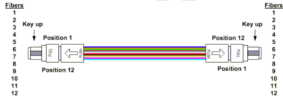
Figure 9 - Type-B:1-1 array patch cord and array cable (key-up to key-up)
