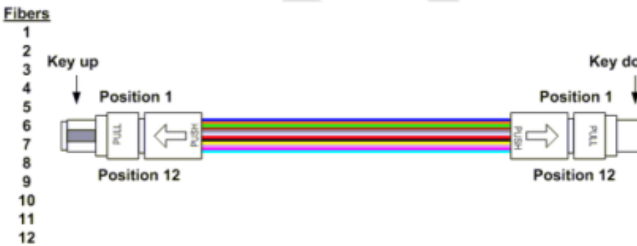
Figure 7 - Type-A:1-1 array patch cord and array cable (key-up to key-down)
